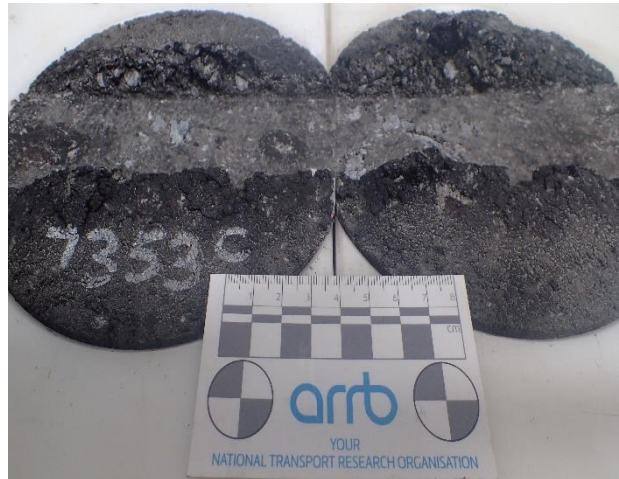
Control asphalt Hamburg top view
