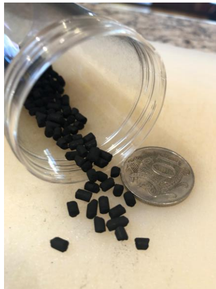
Above: Pearl's carbon char as a powder and right Pearl's test pelletised product using its carbon char and fuels as a binding agent, allowing easy handling and transport – source Company.
