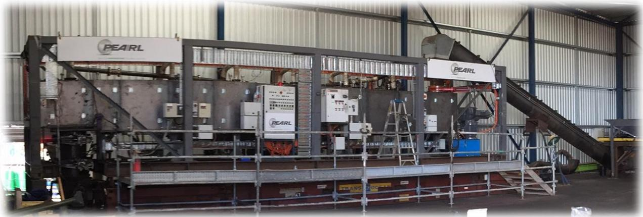
**Fig 2 - Thermal Desorption Unit in Stapylton, QLD**
